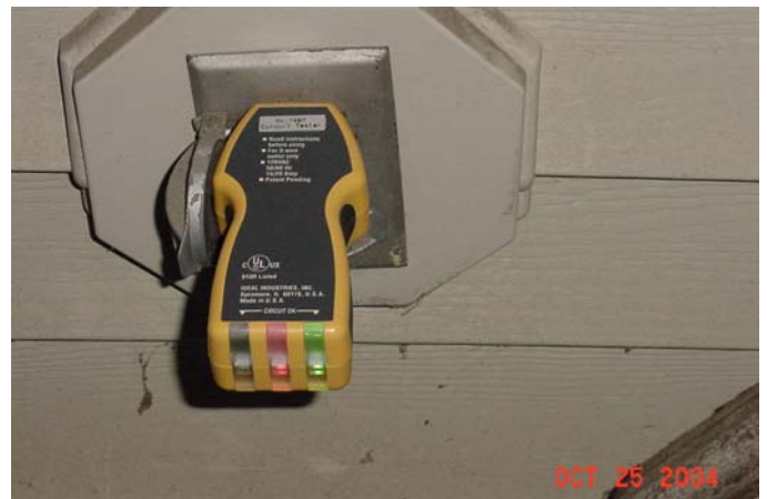
UNSAFE, reversed polarity
